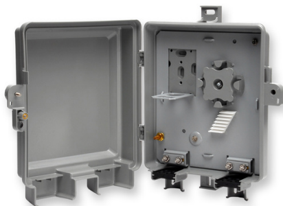
Fiber Transition Housing, FTH-76S, slack routing spool with splice holder, ground post, hex screw
