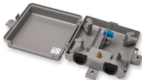
Fiber Transition Housing, FTH-601, 1 LC duplex adapter, ground post, hex security screw, 3 meters slack storage
