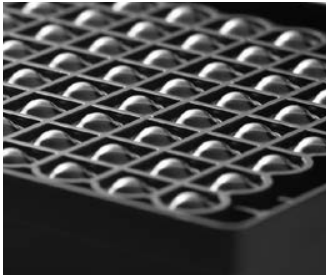
96-well and 384-well round bottom Ultra-Low Attachment microplates enable high-throughput fluorescent spheroid assay screening. The unique microplate underside design shields well-to-well cross-talk.
