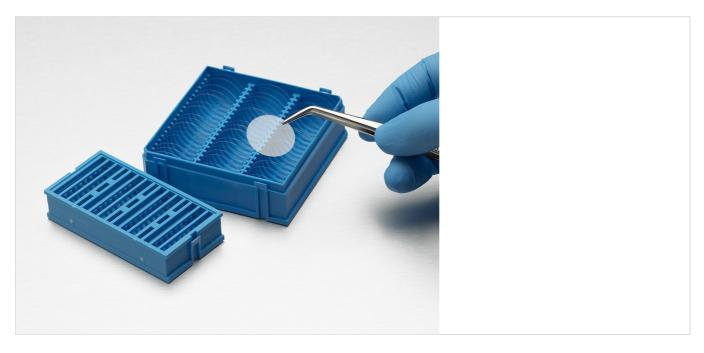
Corning® BioCoat™ 22x22mm #1 German Glass coverslip with a uniform application of human fibronectin. Bulk packed, 60/case. Corning BioCoat products are an ideal solution for enhanced cell attachment and growth of a variety of primary cells and transformed cells in serum-free or serum-containing cultures. Corning offers custom coating capabilities.
